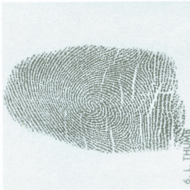
Figure 9.36 The fingerprint from Figure 9.27 compressed at 0.25 bit per pixel or at a ratio of 32 : 1.
